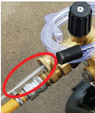
Fig3: High pressure outlet: This is where the high-pressure hose connects.
