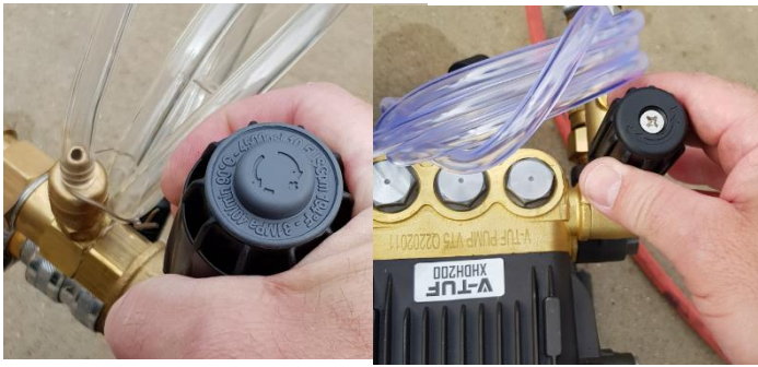
Fig2: Pressure adjustment knob to adjust the pressure on water usage of your machine (these may differ in looks) – turn anticlockwise for a lower pressure and water usage and clockwise for a higher pressure and higher water usage.
