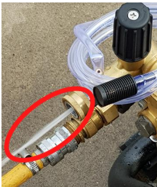
Fig3: High pressure outlet: This is where the high-pressure hose connects. If your machine does not have a Priming/decompression valve, it may be best to start the machine with the high pressure hose off this point, when sucking water from a tank.
